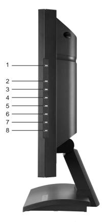
There are 8 keys for user's control including "Enter", "♠", "▼", "Exit", "Mode", "Input" and "*iKey*" and a power switch. The following descriptions are the introduction of these keys & switch.
